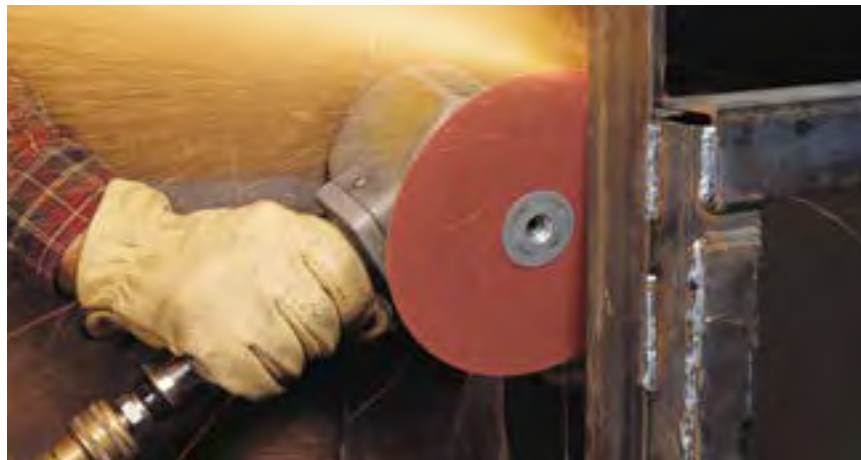
Weld spatter clean-up: 3M™ Fibre Disc 782C
